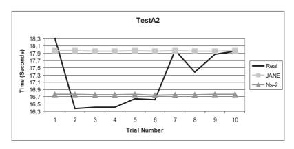
Figure 3: Test A2. Transmission times when transferring 10 times the 10-MB file in Scenario A.
