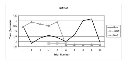
Figure 4: Test B1. Transmission times when transferring 10 times 1-MB file in Scenario B.
