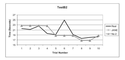
Figure 5: Test B2. Transmission times when transferring 10 times 10-MB file in Scenario B.
